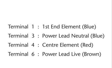
Once repair in completed the toaster should be tested to P.A.T requirements. Dualit also recommends that a residual current device be used to protect the appliance
